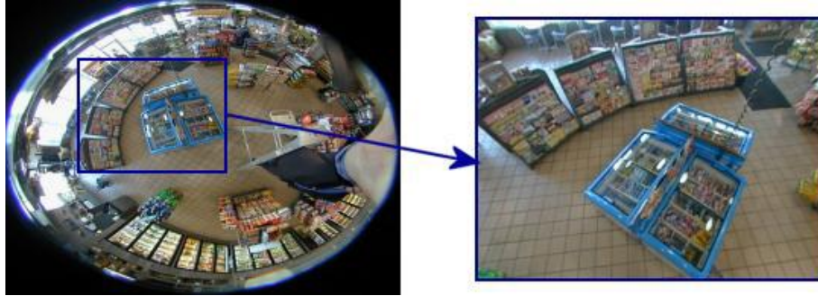
Figure 3: Real-time distortion-free display (left: original image produced by the panomorph lens).
