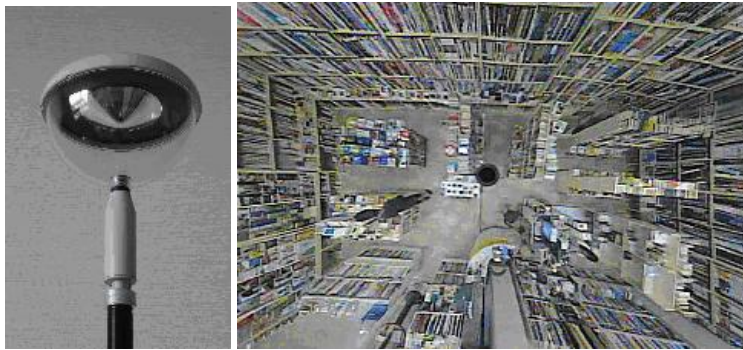
Figure 5: Photograph of the lens with the camera on a pole (left sample image).
